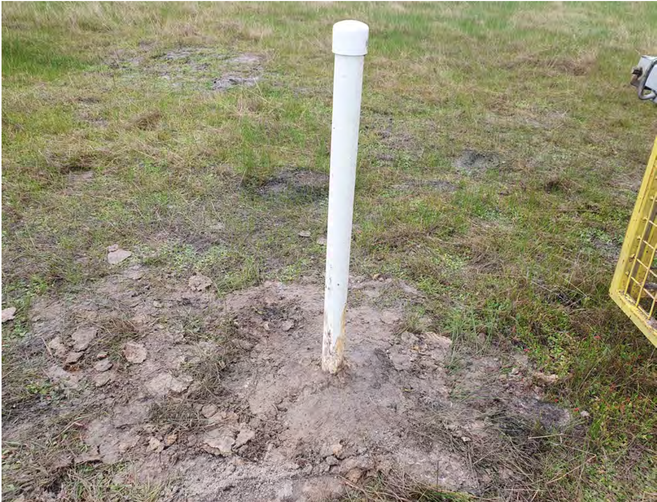
Photo 3: Typical groundwater monitoring well
