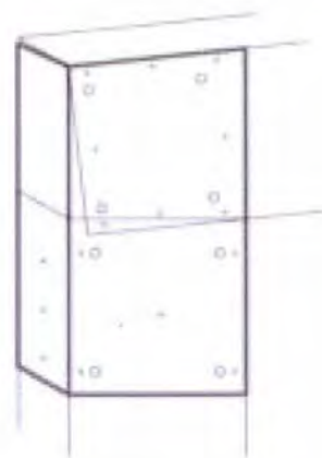
FIXING BOLTS - 8 x M16.30 (8.8) FIXING SCREWS - 16 x 14.20 x 22 HAUNCH PLATE - C300 12deg Reg A+B
