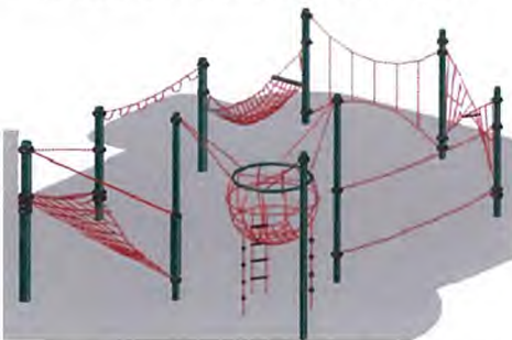
Indicative image of proposed circuit format ropes adventure course. Note: latest draft concept design has one additional triangular net added next to the one shown.
