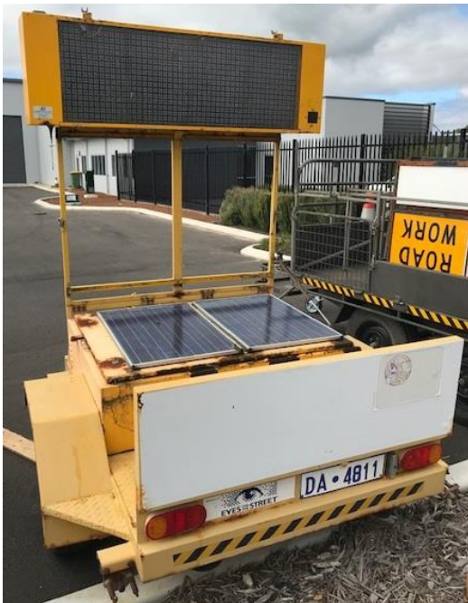
Existing Speed Alert Mobile Trailer
