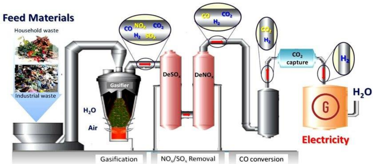
Figure 4: Municipal gasification process (from Demoral, Gunay and Malayao. 2018, 'Energy Use in Municipal Services')
