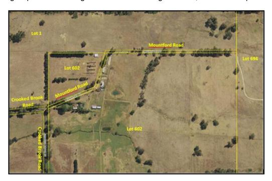
The Master Plan for Road Improvements contained in the Shire's Road Asset Management Plan indicates that Mountford Road should be upgraded to a 4.5 metre wide gravel pavement within a full formation width of 8.5 metres (i.e. full profile consisting of pavement and roadside drains). It is important to note that the road will not be sealed. This standard is adopted due to the rural setting and very low traffic volumes (i.e. less than 20 vehicles per day).
