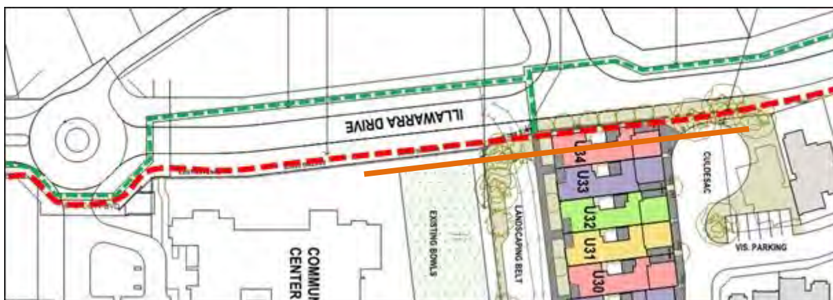
Figure 2: Diagram shows the original location of the footpath in red, the indicated development setback under the Structure Plan in orange and the proposed amended footpath alignment in green.
