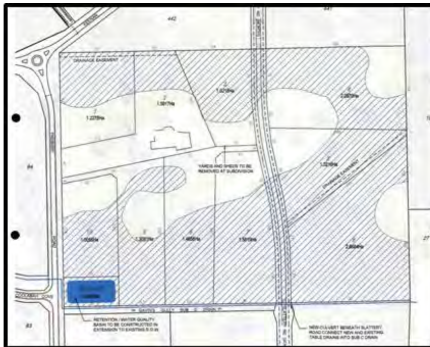
Note: Cross Hatched Areas are 'Building Exclusion Areas' (See Appendix ORD: 12.1A)
