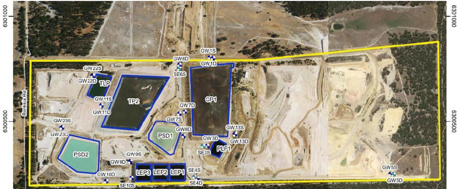
Figure 2: Groundwater Monitoring Bore Locations
