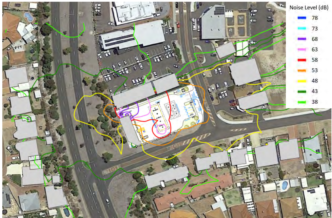
Figure 4 - Forecast L_{A1} night-time noise emission with sources from Table 5 (1.4m above ground level) ( L_{A1} criterion at residences = 53 dB)
