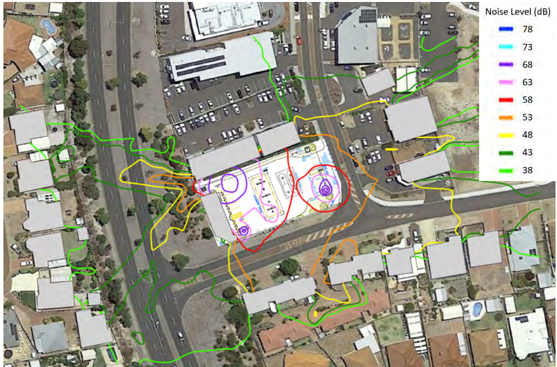
Figure 5 - Forecast Night-time L_{Amax} noise emission – (1.4m above ground level) ( L_{Amax} criterion at residences = 63 dB)
