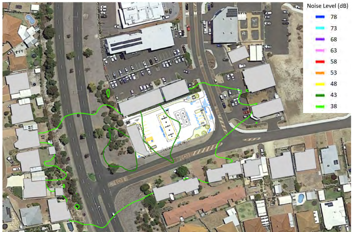
Figure 3 - Forecast L_{A10} night-time noise emission with sources from Table 4 (1.4m above ground level) ( L_{A10} criterion at residences = 43 dB)
