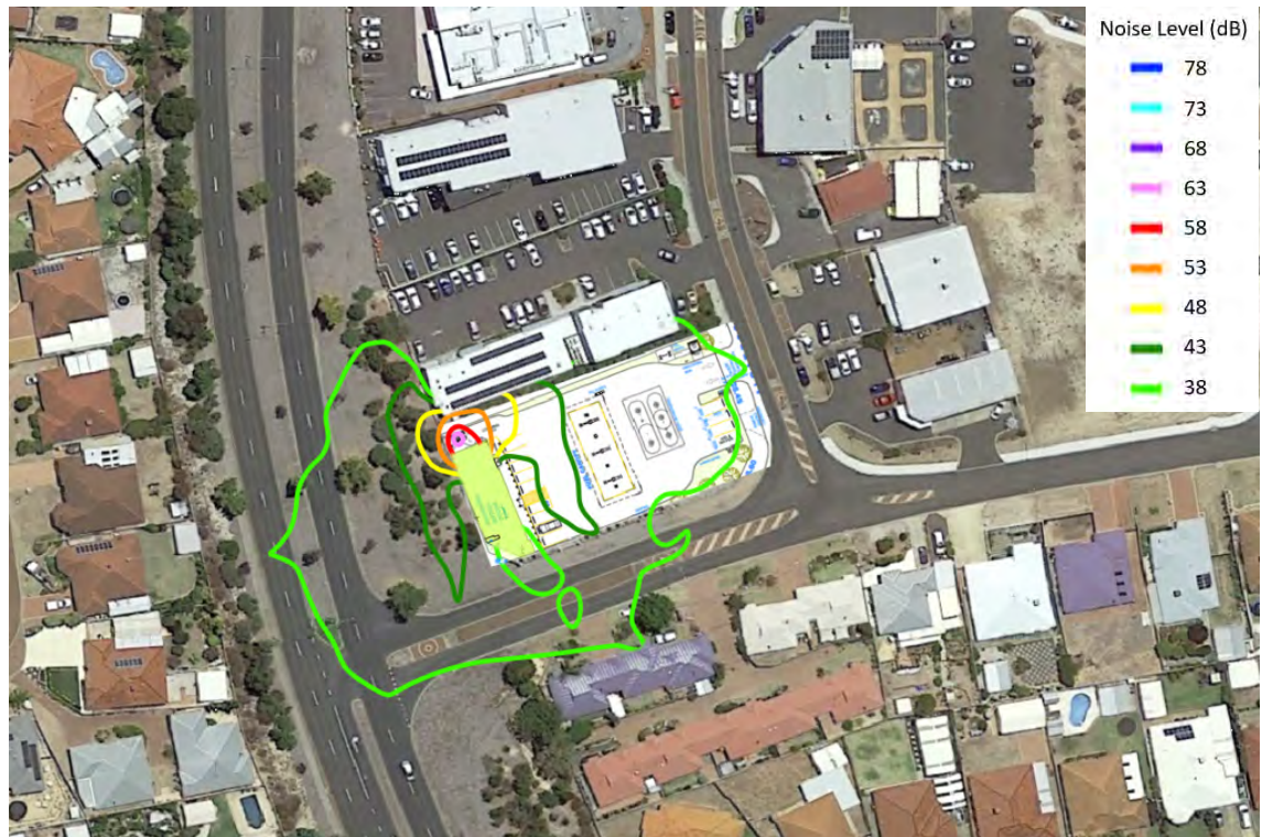
Figure 4 - Forecast LA1 night-time noise emission with sources from Table 5 (1.4m above ground level)
