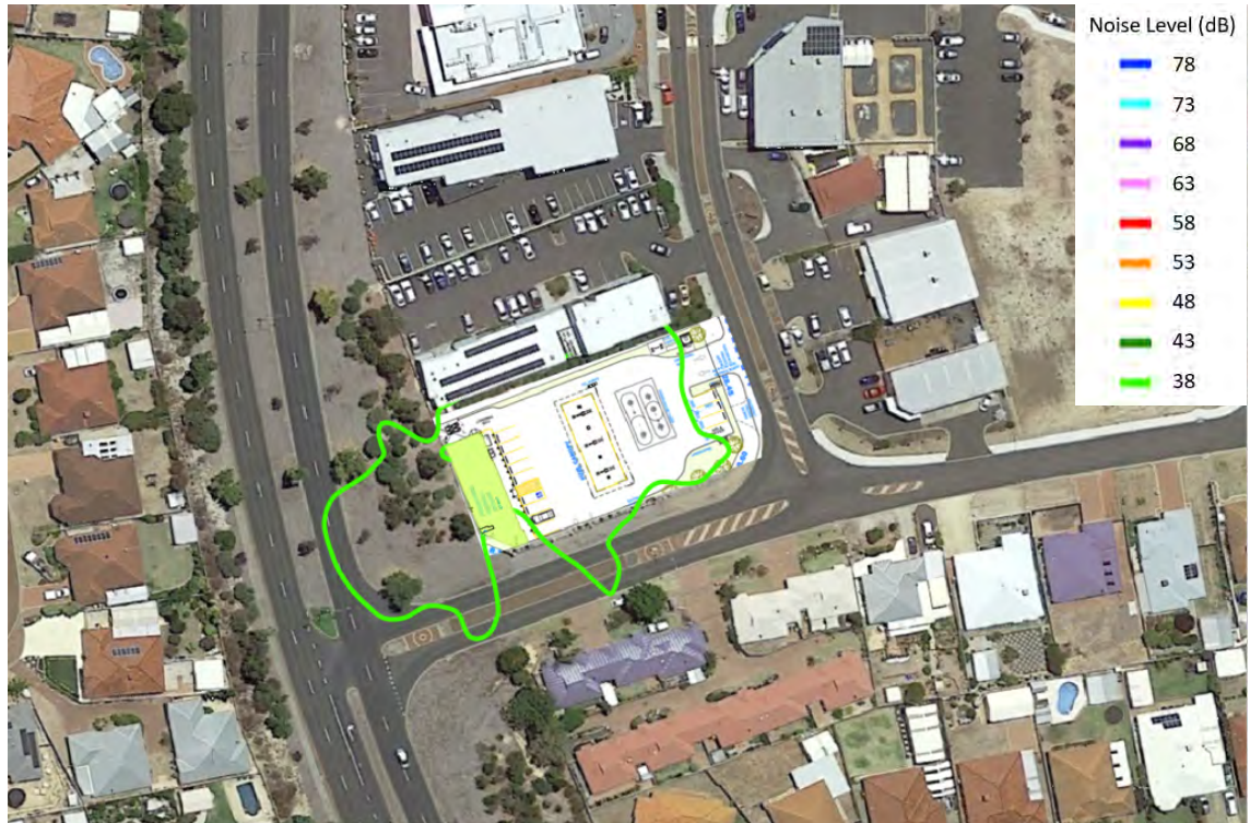
Figure 3 - Forecast LA 10 night-time noise emission with sources from Table 4 (1.4m above ground level)
