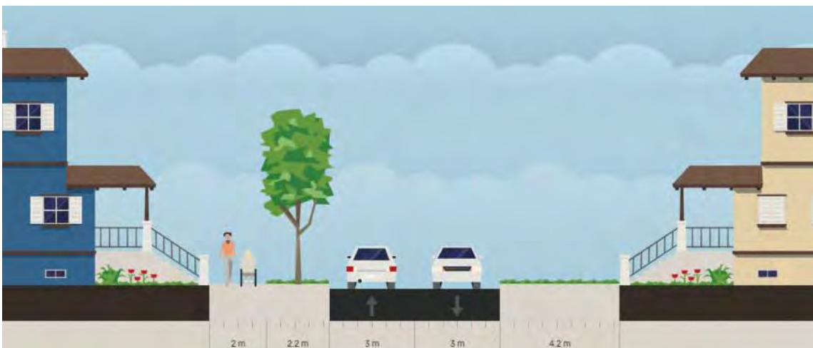
Figure 13 - Typical Access Road Cross-section
