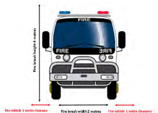
Minimum clearance for fire break in general farming, restricted use and tourist zones
