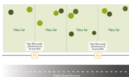
1. Example of a subdivision with no existing network that meets fibre ready requirements
