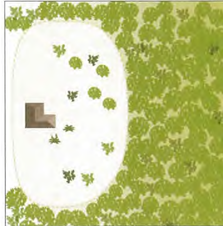
Hazard on three sides APZ
