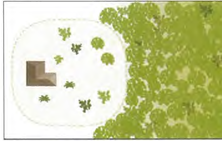
Hazard on one side APZ
