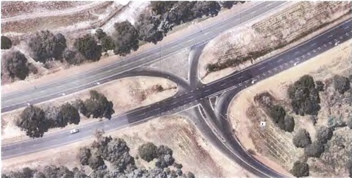
Figure 2.5: Previous intersection geometry - Forrest Highway / Hynes Road
