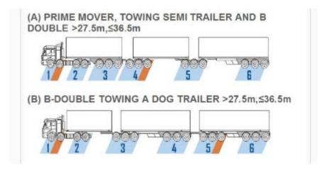
Total length is 36.5 metres and total mass at AMMS Level 3 is 121.5 tonnes (approximately).
