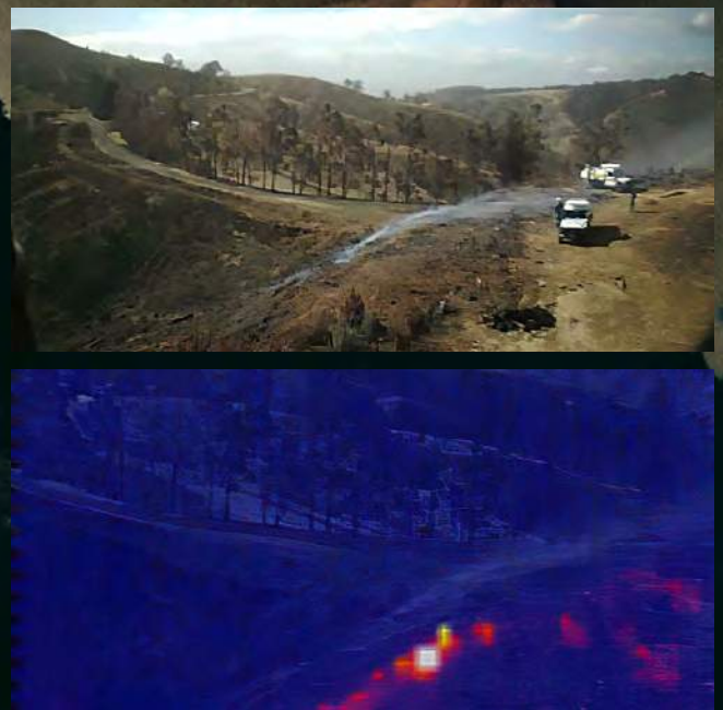
Photo 2-2: Side-by-side thermal and visual image from the LVIN showing the heat sources(s) detected and crews onsite for the same fire shown above in March 2019. This autonomous detection sends an alert to any individual or group who have set up alarm configurations. Provided by Latrobe City Council on 21 July 2020.
