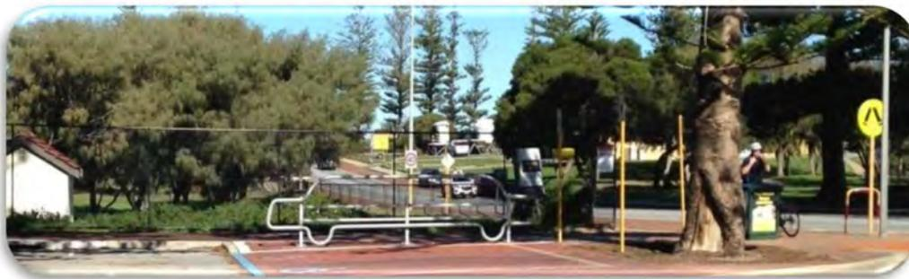
Short stay EoT facilities should generally be in the form of simple u-rails or other design, which facilitates the secure parking of a bicycle. In accordance with Austroads Guidelines, these should be located approximately every 30 metres along 'main street' type shopping strips and in small clusters at the entrances to shopping centres and other significant destinations.
