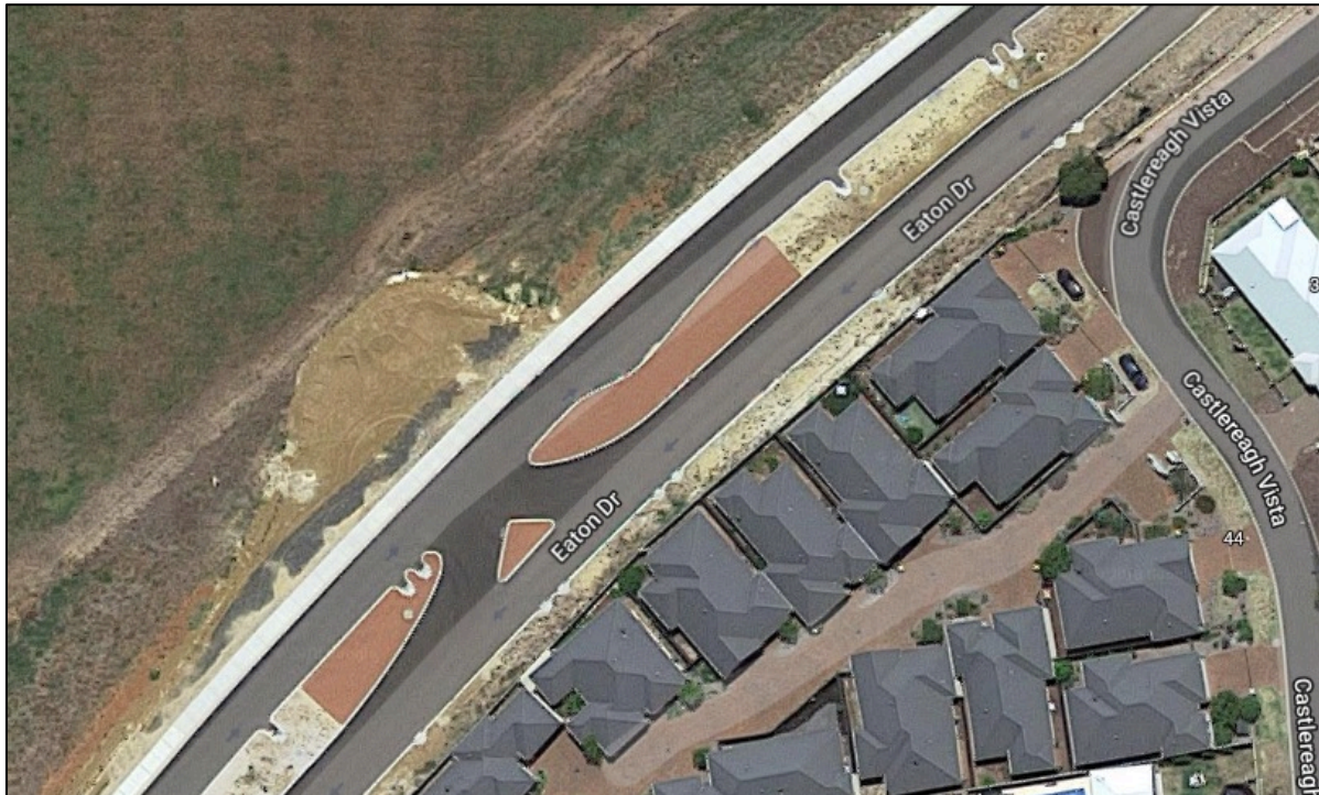
Figure 2 Seagull Intersection Treatment
